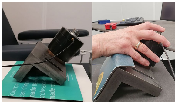
Figure 1. Photographic images showing the tactile actuator. The right picture demonstrates the placement of the right index finger on the mini-shaker.
